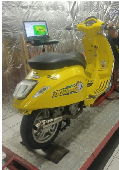
Figure 1. Installation of the Vespa Sprint I-Get 150 ABS Motorcycle on the Dynamometer
