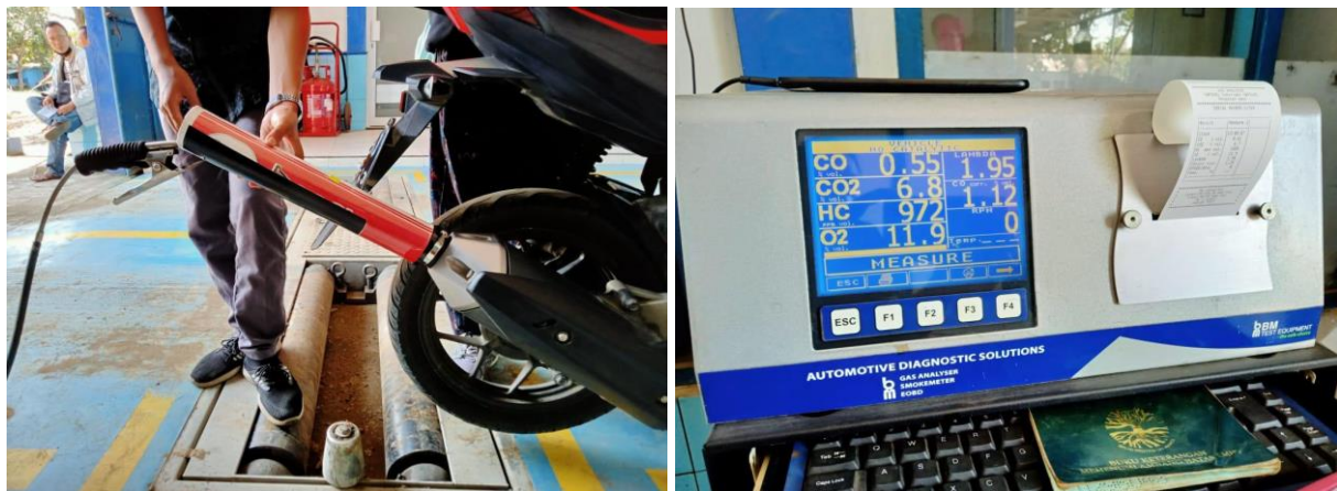
Figure 5. Emission Test at the Cilacap District Transportation Office
