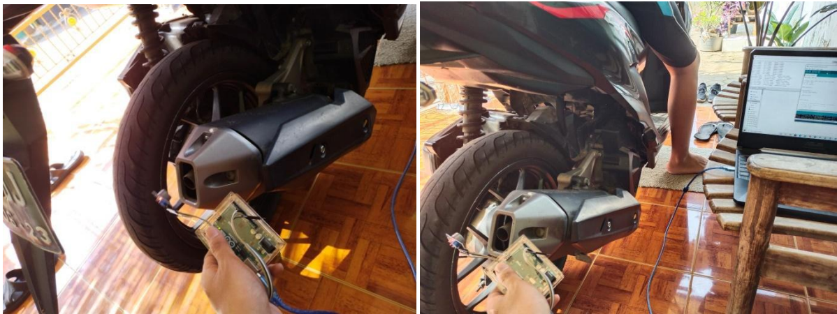
Figure 4. Smoke and CO test using the MQ-135 sensor
