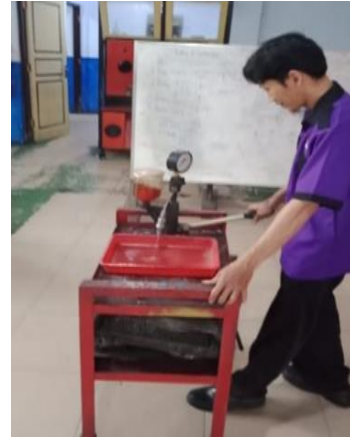
Figure 2. Graph of Injector Testing using Pressure Tester Nozel
