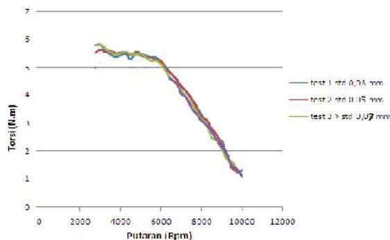
**Figure 3.** Engine Torque Testing Chart
