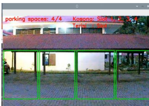
Figure 6. Parking Slot Coordination Box
