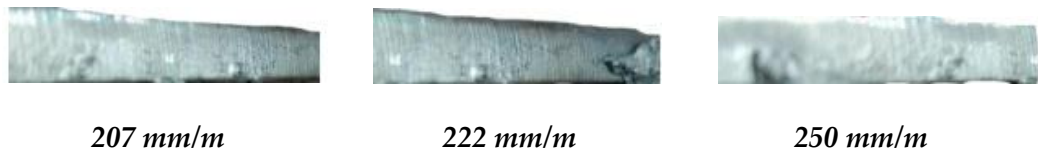
Figure 5. Visual results of cutting 5 mm steel
