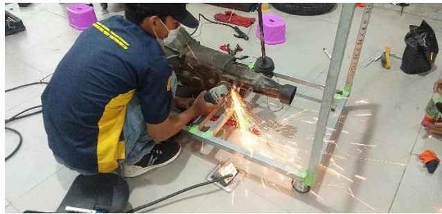
Figure 7. Proses Cleaning of excess welds and Iron
