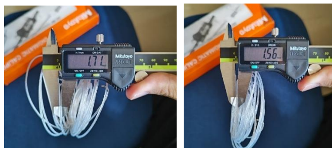
Figure 3. Measurement of PET filament diameter
