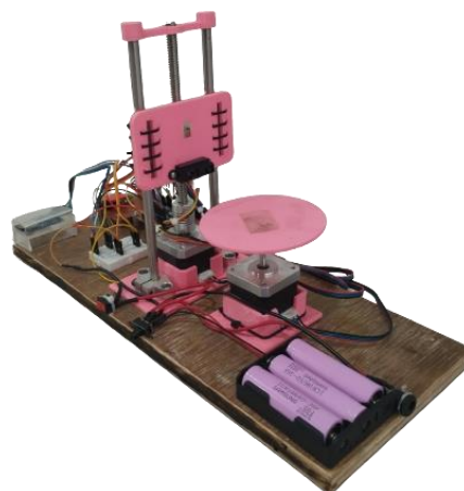
Figure 6. Assembled 3D scanner
