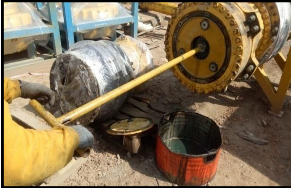
Figure 5. Trial Service Tools Remove & Install Drive Shaft
