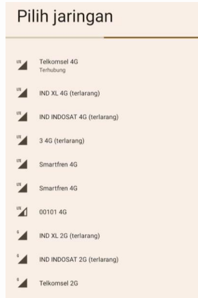
Figure 12. 4G Network Display from USRP B210 has been successfully detected with network name “00101 4G”
