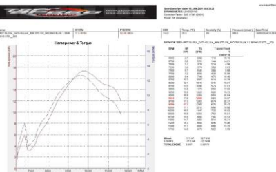
Test results of Packing Block with Thickness 1.3 mm
