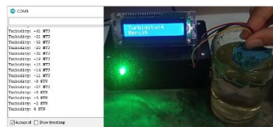
Figure 5. Test Results of the Clean Water Turbidity Sensor Measurement System
