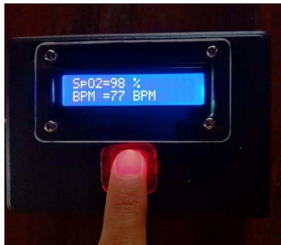
Figure 4. Display of measurement results on a 16x2 LCD
