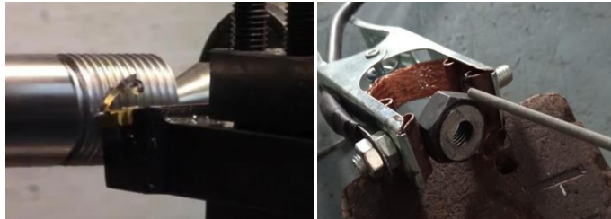
Figure 7. Threading & welding of bracket nut
