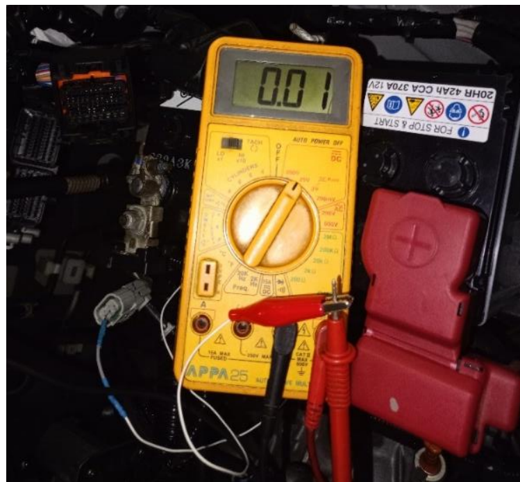
Figure 7. Circuit A2 voltage
