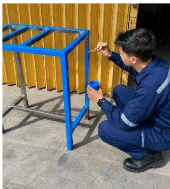
Figure 6. Painting Process of the Media Frame
