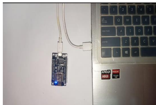
Figure 10. Nodemcu Connected by USB To A Laptop
