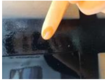
Figure 8. The Clear Coat Has Dried Adhesion
