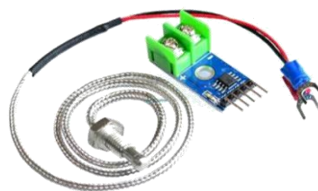
Figure 5. Thermocopel Type K dan max 6675
