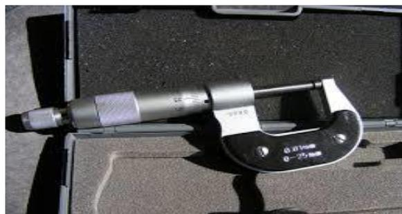
**Gambar 5.** Mikrometer Skrup
