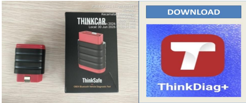
Gambar 2. Scanner THINKCAR ThinkSafe OBD-II Bluetooth Vehicle Diagnostic Tool dan aplikasi Thinkdiag
